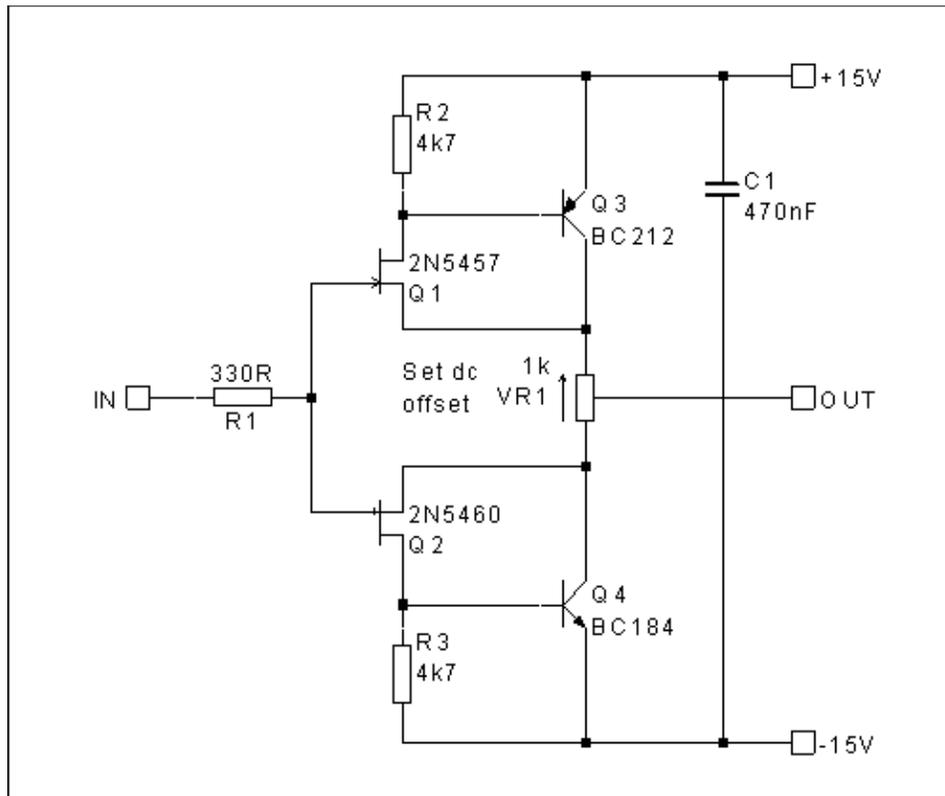
The bipolar-FET symmetrical compound source follower circuit works extremely well, with negligible steady state or transient distortion.
